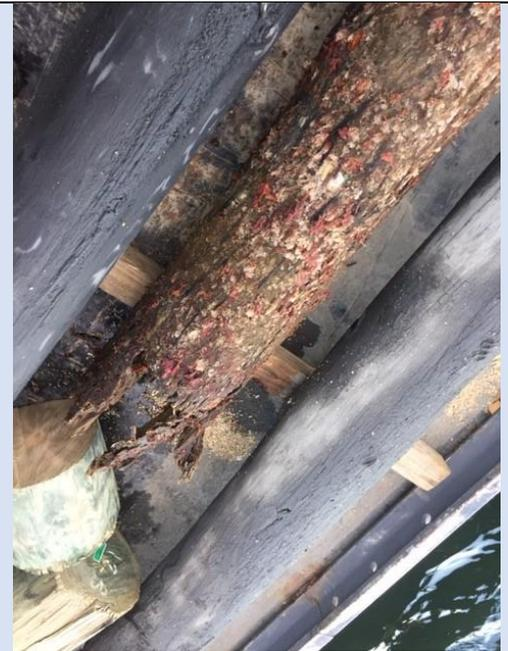
*Pile Pulled from Pier. Broken stub left under the mudline.*
